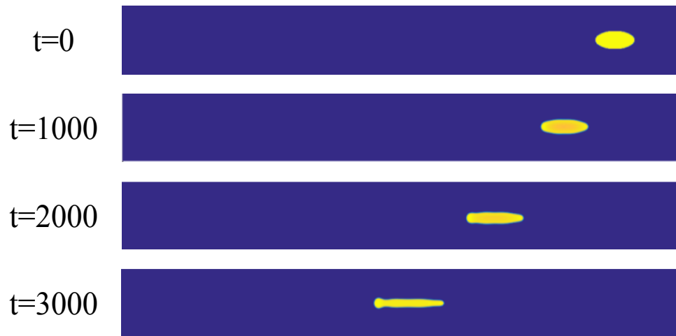
Figure 5.5. Pore migration simulation using Eq. (4.11) and starting from a 5:1 ellipsoid Snapshots of a simulation showing pore migration when using Eq. (4.11). The images are arranged top-to-bottom and correspond to 0, 1000, 2000, and 3000 simulation steps, respectively. These images were taken from a simulation that used the larger grid (1024×128).
